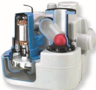
**SEWPAC** - Sewpac range of packaged sewage ejector stations have been developed for the disposal of sewage from single dwellings, or single toilet/basin installations. The package comprises various sizes of one piece polyethylene tanks, a single/duplex sewage pump fitted with vortex impellers, a single or three phase IP68 motor, and a sheet steel IP54 wall mounted control panel.
